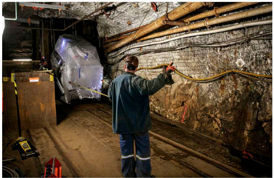
LZ's central detector was assembled in a surface cleanroom and moved to the nearly mile-deep campus at the Sanford Underground Research Facility. The underground location shields the experiment from cosmic rays. (Photo Credit: Matthew Kapust/Sanford Underground Research Facility)
