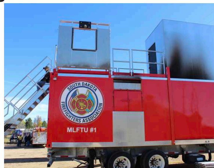
The MLFTU open up to multiple levels for firefighter to train on different levels. The upper deck has a tie down ring allowing for practice rappelling down the side of the trailer. The Firefighters Association has two units that can be made available anywhere in the state at the same time. Longbrake photo
