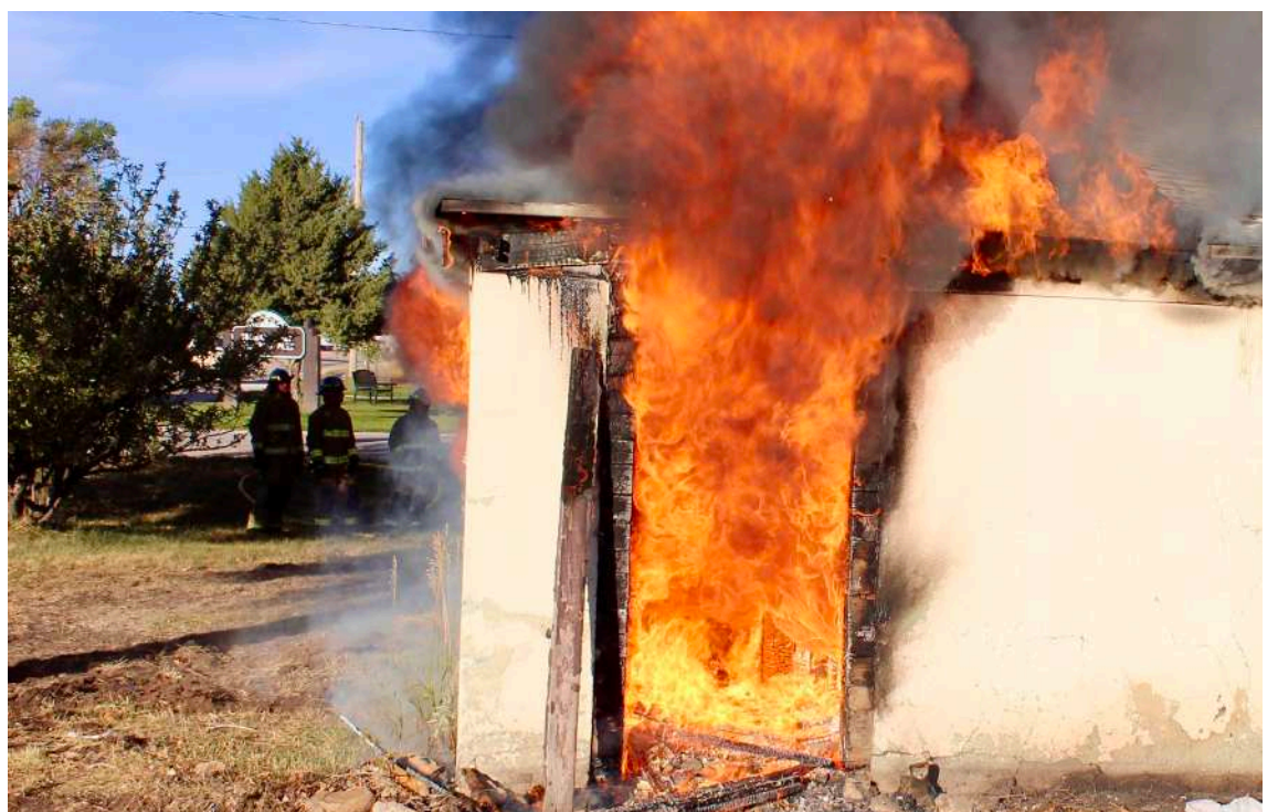
Watching a bidirectional flow pattern develop. It occurs when smoke and air move in opposite directions through the same opening.
