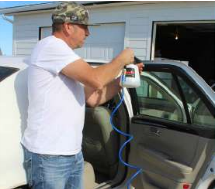
The "Tornado" is a specialty steamer Berger uses to clean door gaskets and consoles in vehicles. - Brunner photo
