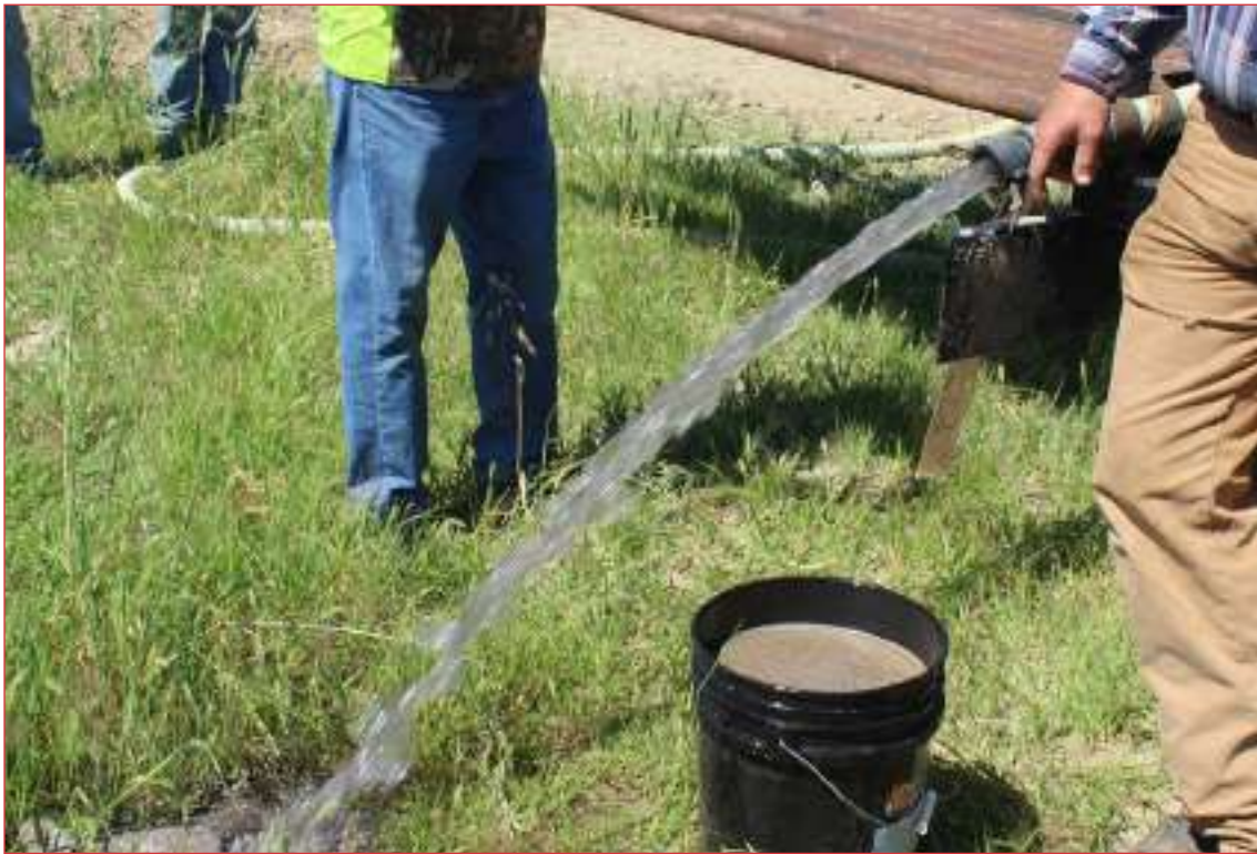
The water from the Castle Rock well north of Newell flowed out at 87 gallons per minute, measured by professionals from Keller Drilling of Lemmon. - Brunner photo
