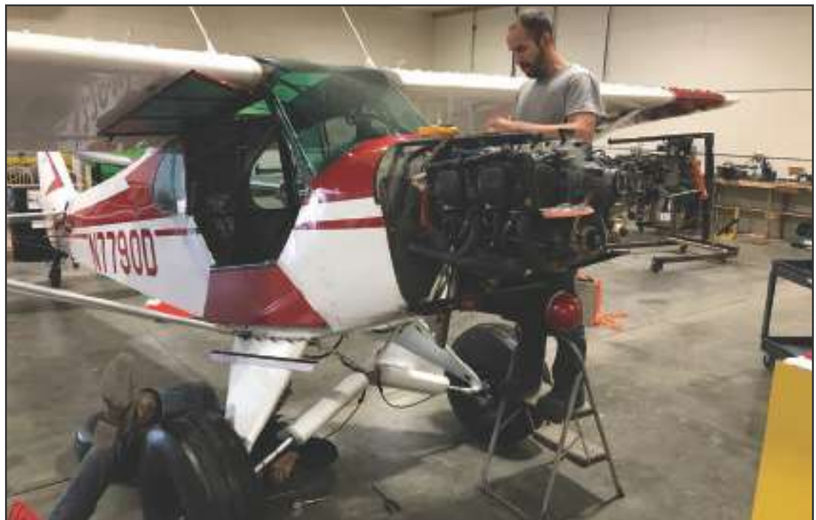
KEEPING ‘EM FLYING - Aircraft mechanics Nate Kalkbrenner (right) works on the engine of a Piper Super Cub along with James Kahler (left) who works underneath on a strut inside the hanger at the Belle Fourche Flight Center.
