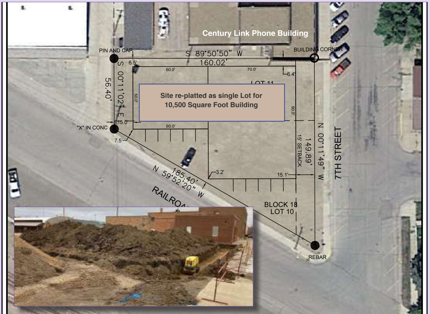
The Center of the Nation Wool's site plan of the Wool storage building that is being constructed at the corner of 7th and Railroad Streets. The inset photo of foundation excavation underway by Albright Construction. Beacon Photo
